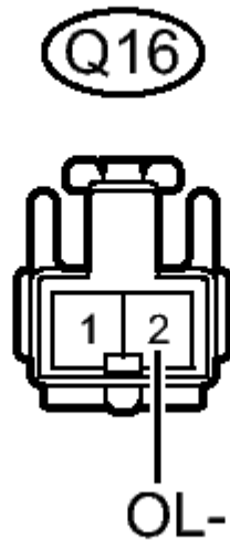
Fig. 46: Checking Q16 Limit Switch Assembly (Outward Slide Origin Point Switch) Courtesy of TOYOTA MOTOR SALES, U.S.A., INC.
