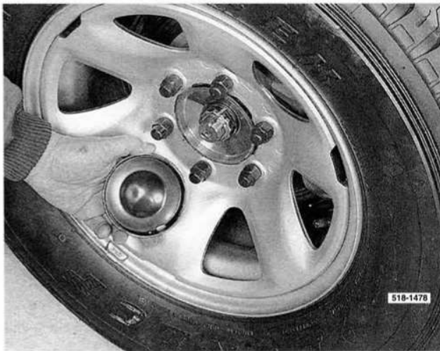
Dust cover removed showing the drive shaft end components.
