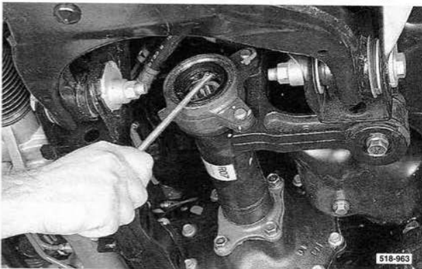
Removing the drive shaft oil seal from the final drive housing.
