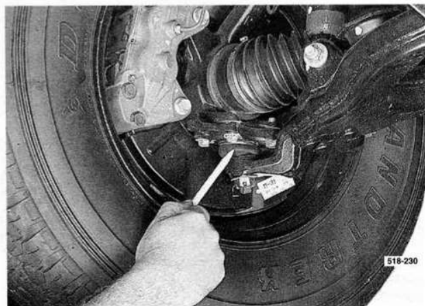
Check the lower ball joint for deterioration and wear.
