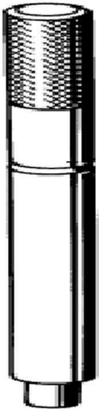
Fig. 13: Identifying 11 2 300 Plug Mandrel Courtesy of BMW OF NORTH AMERICA, INC.
