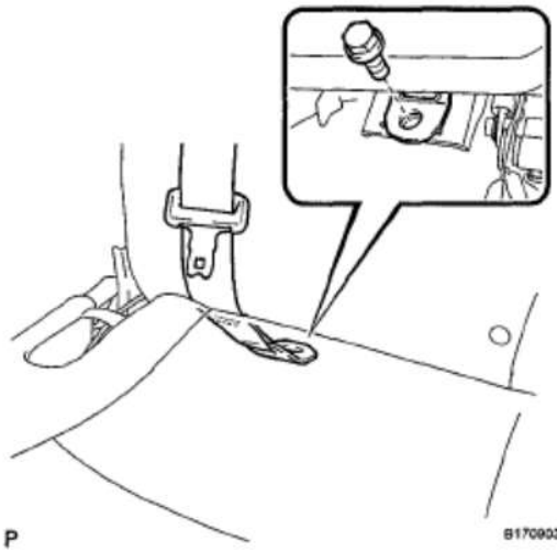
Fig. 91: Identifying Rear Center Seat Outer Belt Assembly With Bolt Courtesy of TOYOTA MOTOR SALES, U.S.A., INC.
