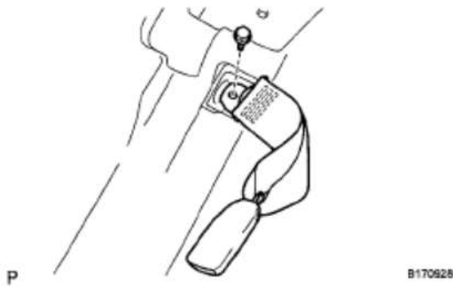
Fig. 86: Identifying Rear Center Seat Inner Belt Assembly With Bolt Courtesy of TOYOTA MOTOR SALES, U.S.A., INC.
