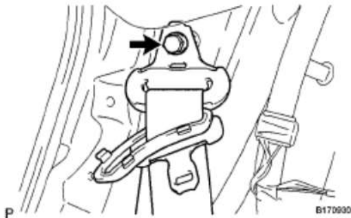
Fig. 83: Identifying Shoulder End Of Rear No. 2 Seat Outer Belt Assembly With Bolt Courtesy of TOYOTA MOTOR SALES, U.S.A., INC.
