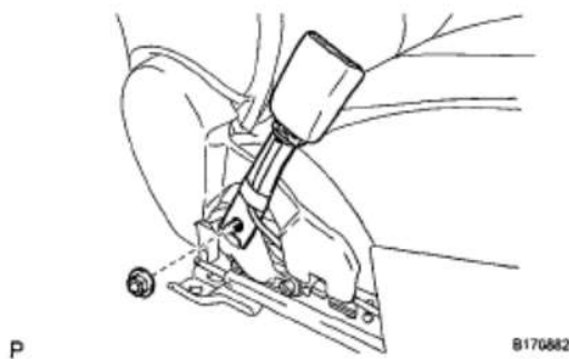
Fig. 18: Identifying Front Seat Inner Belt Assembly Nut Courtesy of TOYOTA MOTOR SALES, U.S.A., INC.
