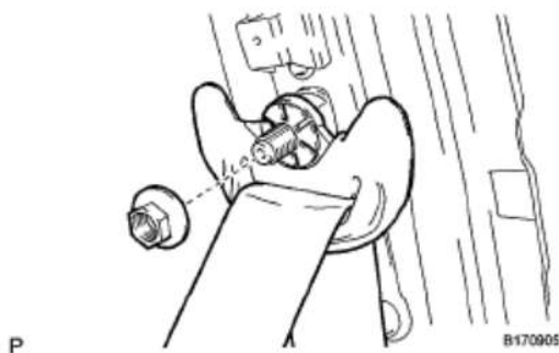
Fig. 25: Identifying Shoulder Anchor Of Front Seat Outer Belt Assembly Courtesy of TOYOTA MOTOR SALES, U.S.A., INC.
