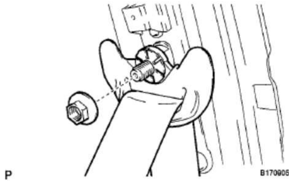
Fig. 33: Identifying Front Seat Outer Belt Assembly Bolts Courtesy of TOYOTA MOTOR SALES, U.S.A., INC.
