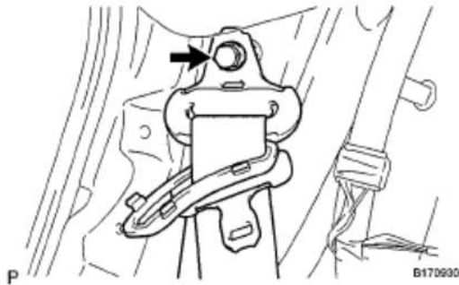
Fig. 80: Identifying Shoulder End Of Rear No. 2 Seat Outer Belt Assembly With Bolt Courtesy of TOYOTA MOTOR SALES, U.S.A., INC.
