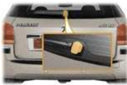
Opening the rear screen of the 407 SW
