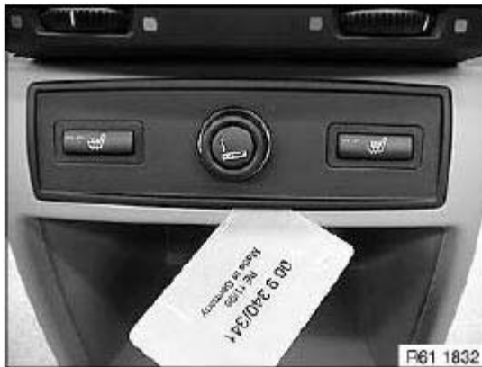
Fig. 182: Unclipping Trim With Special Tool 00 9 340 Courtesy of BMW OF NORTH AMERICA, INC.
