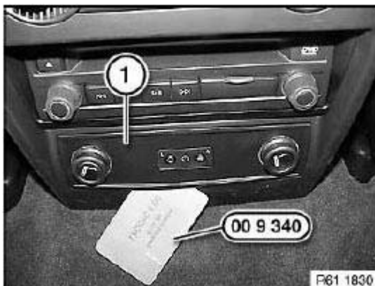
Fig. 192: Unclipping Trim With Special Tool 00 9 340 Courtesy of BMW OF NORTH AMERICA, INC.
