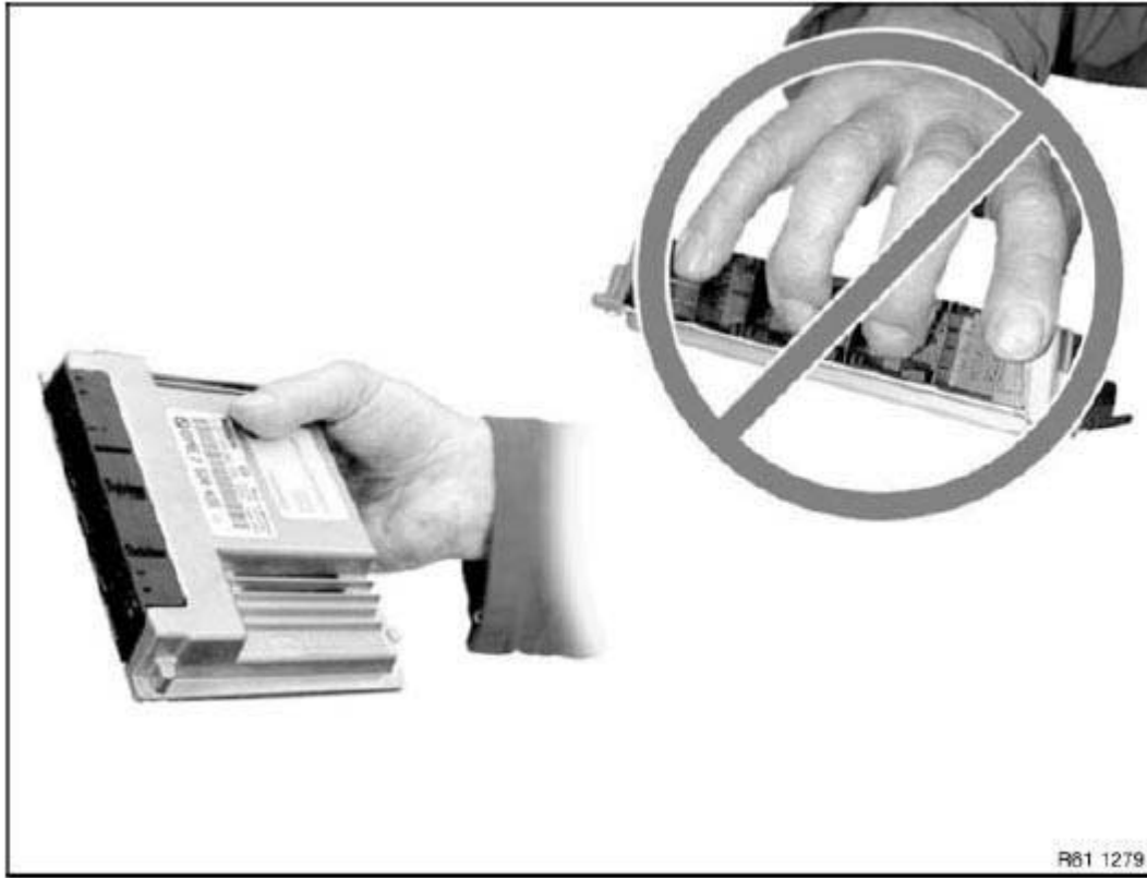
Fig. 234: Precaution For Touching Pins Or Multi-Pin Connectors Directly Courtesy of BMW OF NORTH AMERICA, INC.
