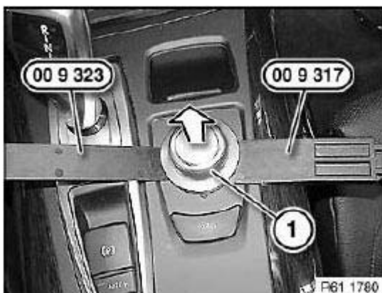
Fig. 196: Removing Knob For Controller
