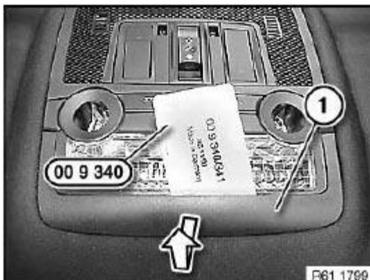
Fig. 178: Levering Out Trim With Special Tool 00 9 340 Courtesy of BMW OF NORTH AMERICA, INC.
