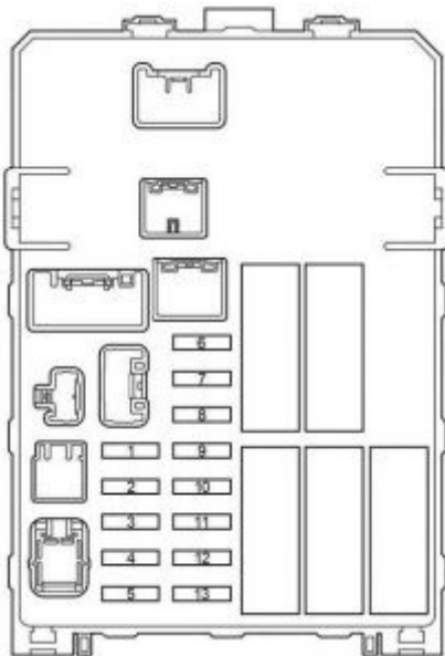
Toyota Fourtour – fuse box diagram – passenger compartment
