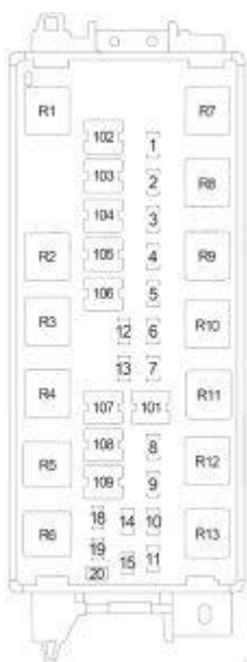
Chevrolet Voyager – fuse box diagram – engine compartment
