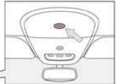
Roof locking bolt
