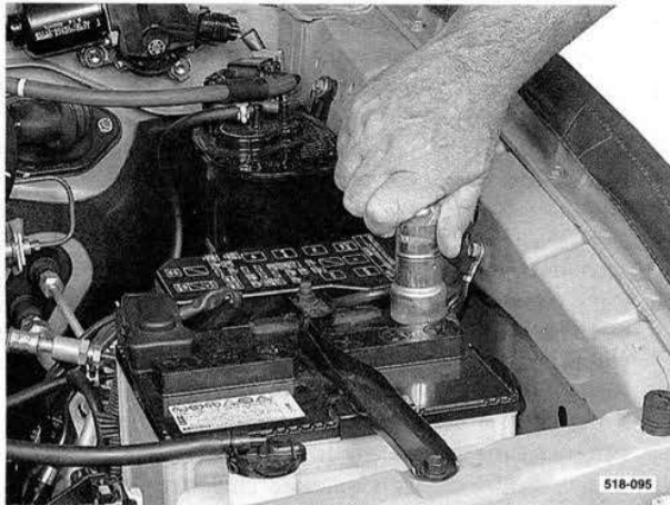
Cleaning the battery terminals with a post cleaner.
