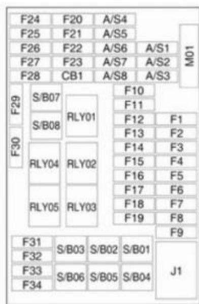
Vauxhall Mokka – fuse box – instrument panel
