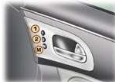
M. Adjustments memorisation. 1. Recall of the first position. 2. Recall of the second position.
