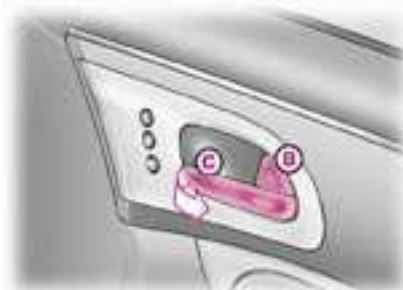
Opening the doors from inside
