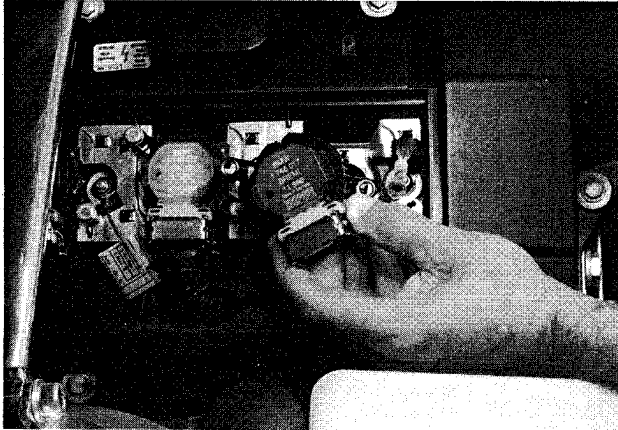
Fig. 12. Ignition coil being removed from spark plug on M52 engine.
