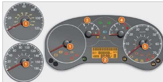
Instrument panel with level 2 display
