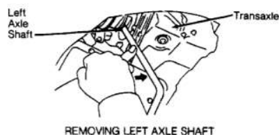
Fig. 13: Removing Left Axle Shafts (Camry) Courtesy of Toyota Motor Sales, U.S.A., Inc.
