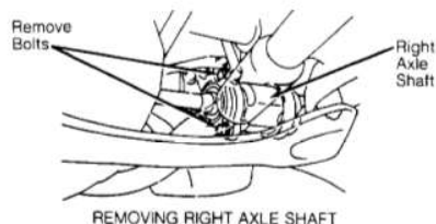
Fig. 18: Removing Right Axle Shafts (Celica) Courtesy of Toyota Motor Sales, U.S.A., Inc.
