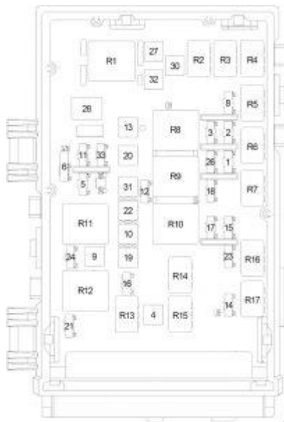
Chrysler Voyager – fuse box diagram
