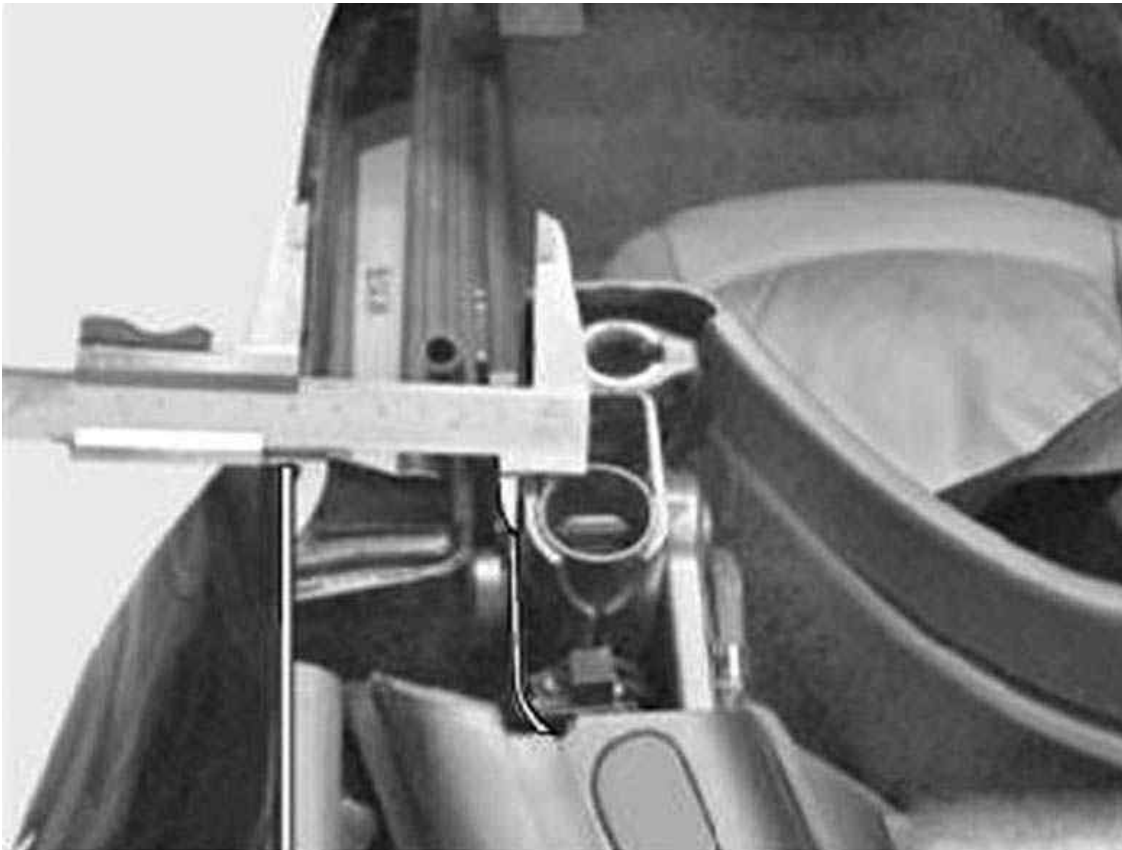
Fig. 8: Measuring Gap Between Inside Edge Of Side Panel & Main Bearing Courtesy of BMW OF NORTH AMERICA, INC.
