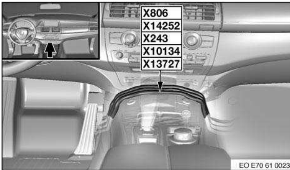
Fig. 27: On Floor, Under Center Of Dash Courtesy of BMW OF NORTH AMERICA, INC.
