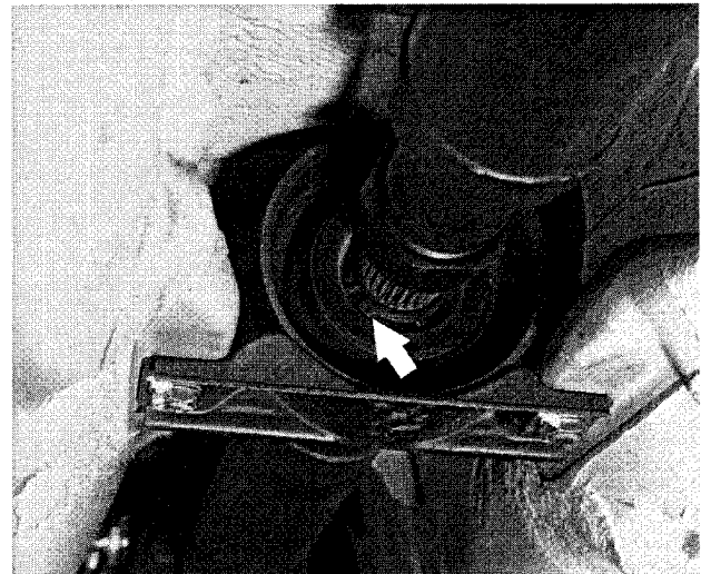
Fig. 10. Center bearing circlip (arrow) to be removed. Driveshaft shown installed.
