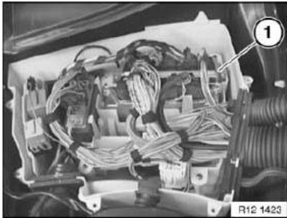
Fig. 34: Identifying DME Control Unit Courtesy of BMW OF NORTH AMERICA, INC.
