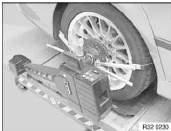
Fig. 17: Identifying Quick-Clamping Holder/Quick-Clamping Unit Courtesy of BMW OF NORTH AMERICA, INC.
