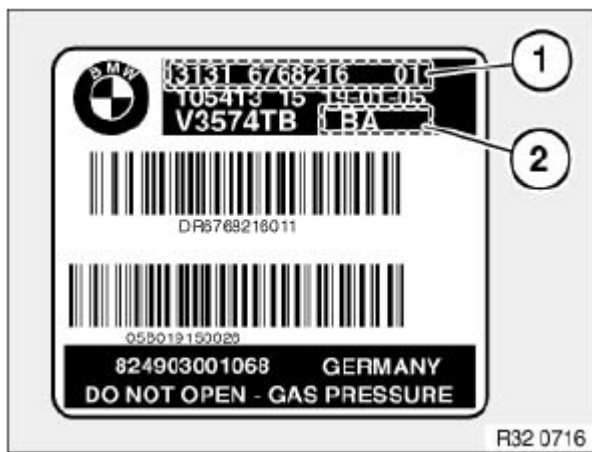
Fig. 14: Identifying Spring Strut/Shock Absorber Label Courtesy of BMW OF NORTH AMERICA, INC.
