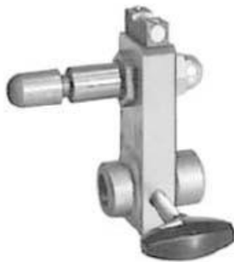
Fig. 22: Identifying Spoiler Adapter Courtesy of BMW OF NORTH AMERICA, INC.
