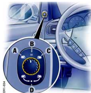
A - Door mirror setting – driver's side B - Heat door mirror C - Door mirror setting – passenger's side D - Fold in door mirrors
