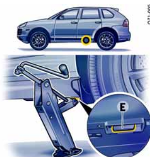
Vehicles with running board Rear jacking point
