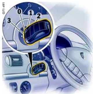
Ignition lock positions: 0 - Initial position 1 - Ignition on 2 - Start engine 3 - Ignition off
