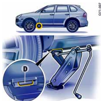
Vehicles with running board Front jacking point
