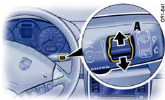
Rain sensor rotary switch
