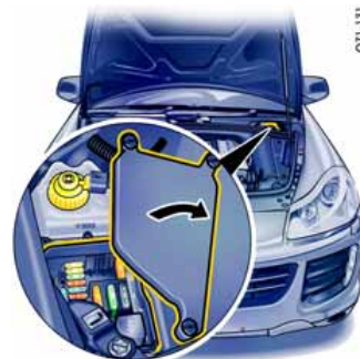
Fuse box in engine compartment
