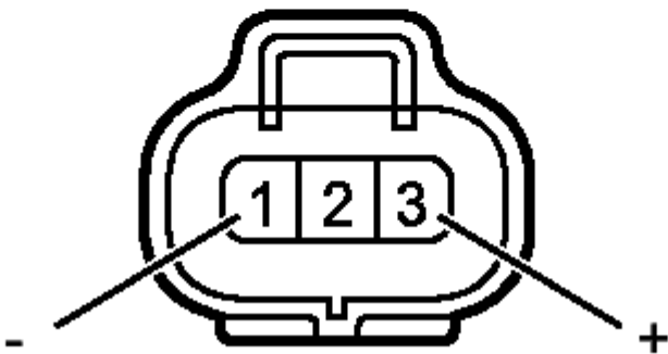
Fig. 265: Air Conditioner Pressure Sensor Connector End View Courtesy of TOYOTA MOTOR SALES, U.S.A., INC.
