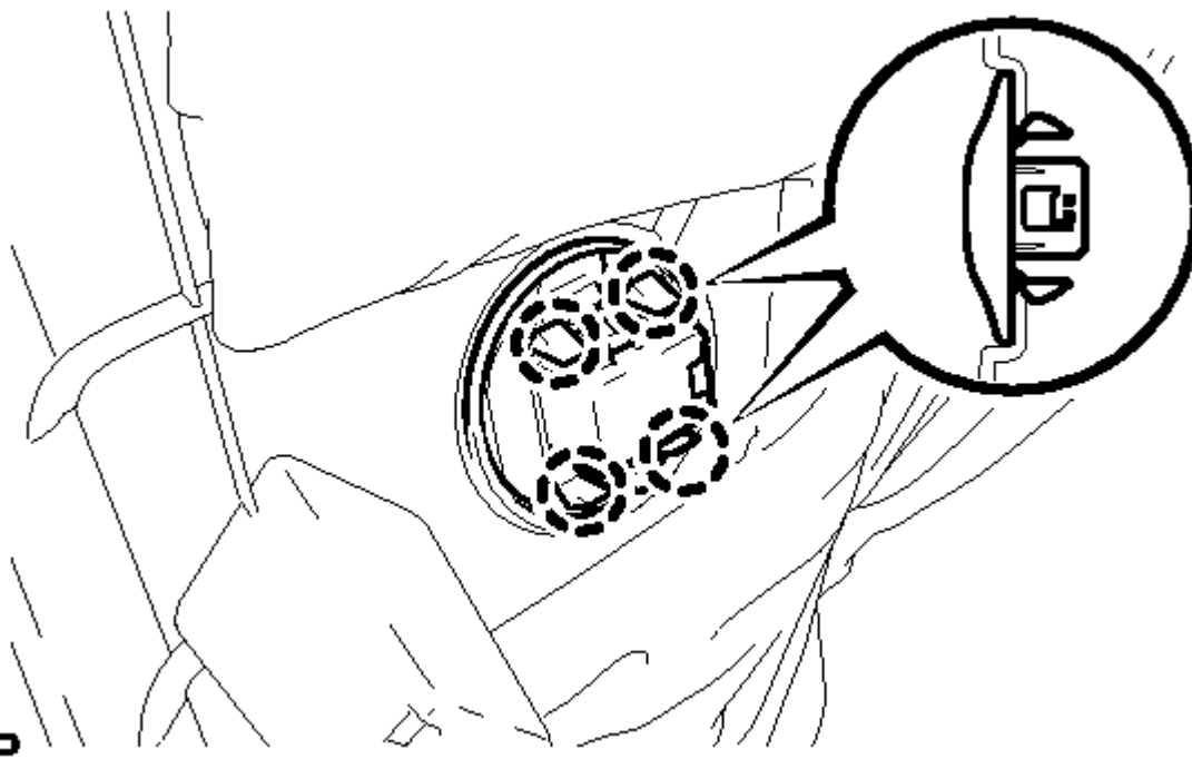
Fig. 244: Identifying Cooler (No. 2 Room Temperature Sensor) Thermistor & Claws
