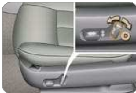
D. Seat back angle adjustment.
