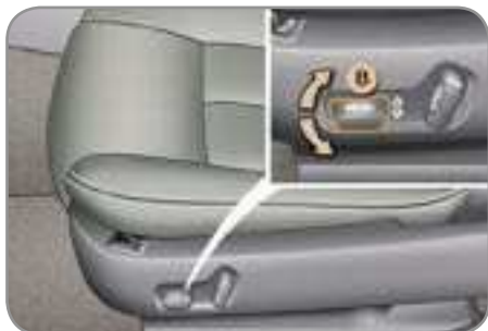
B. Seat cushion angle adjustment.
