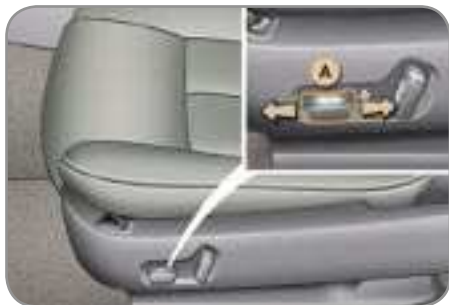
A. Forwards-backwards adjustment.
