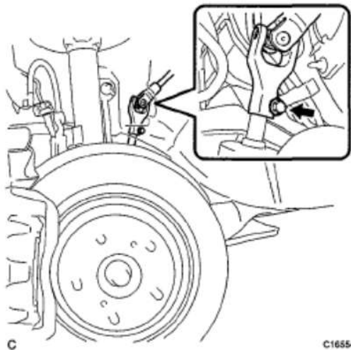
Fig. 80: Identifying Steering Intermediate Shaft Sub-Assembly And Bolt Courtesy of TOYOTA MOTOR SALES, U.S.A., INC.
