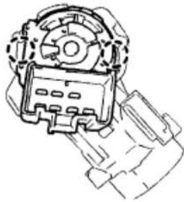
Fig. 62: Identifying Ignition Or Starter Switch Assembly Claws Courtesy of TOYOTA MOTOR SALES, U.S.A., INC.
