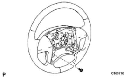
Fig. 102: Identifying No. 2 Steering Wheel Ornament And Screw Courtesy of TOYOTA MOTOR SALES, U.S.A., INC.
