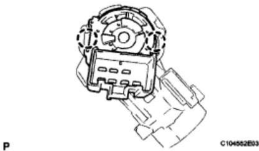
Fig. 66: Identifying Ignition Or Starter Switch Assembly Claws Courtesy of TOYOTA MOTOR SALES, U.S.A., INC.
