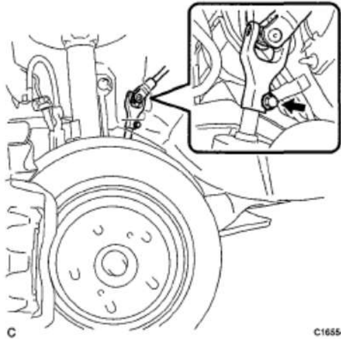
Fig. 47: Identifying Steering Intermediate Shaft Sub-Assembly And Bolt Courtesy of TOYOTA MOTOR SALES, U.S.A., INC.
