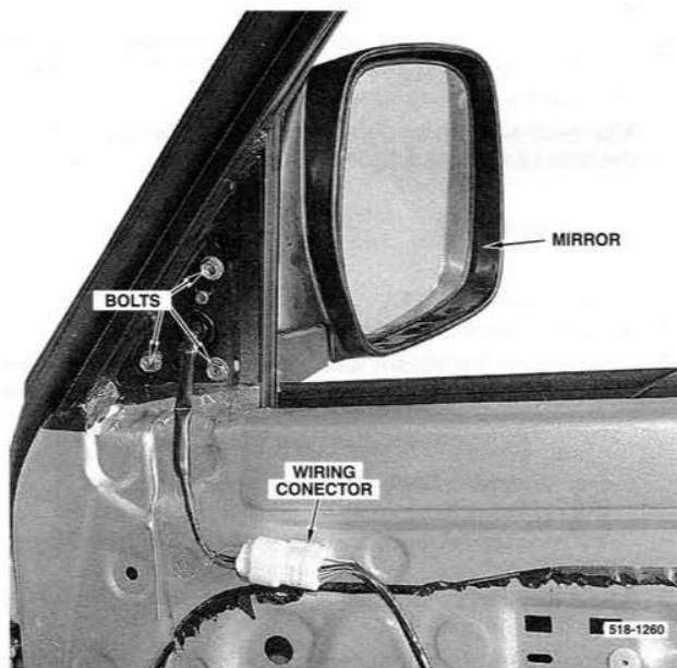
Exterior mirror installed, with trim panel and mirror cover removed.
