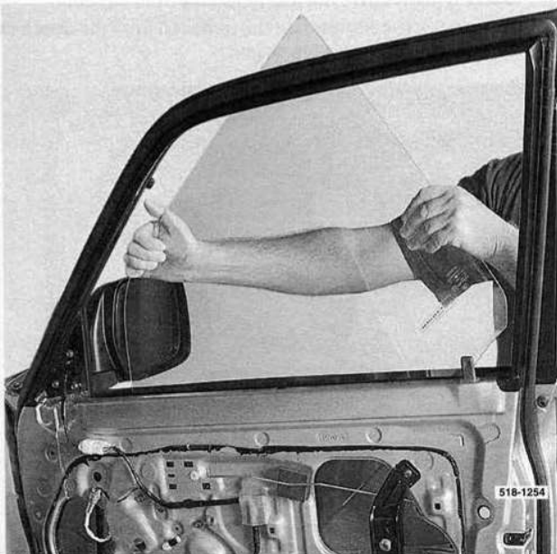
Removing the window glass from the door.
