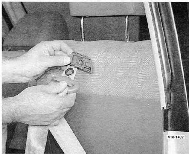
Ensure that the top seat belt anchor is installed correctly to the lock on models with height adjustable seat belts.
