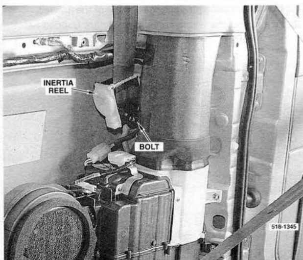
Location of the third seat inertia reel retaining bolt, shown with the rear quarter trim panel removed.
