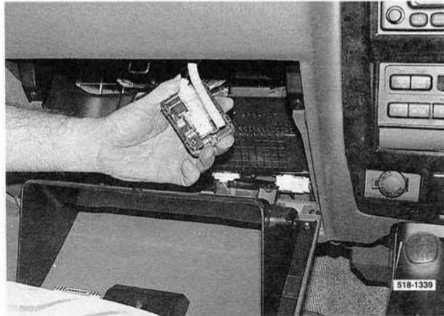
Disconnecting the passenger side airbag connector.
