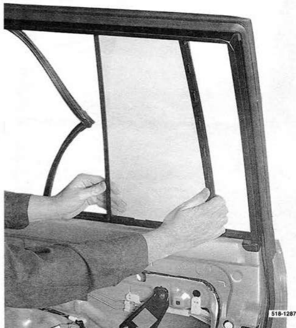
Removing the quarter window glass from the door.
