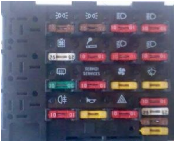
Fiat Uno – fuse box diagram – auxiliary fuse
