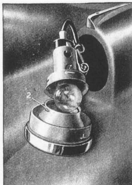
Fig. 49.—SIDE LAMP. 2. Spring catch.
