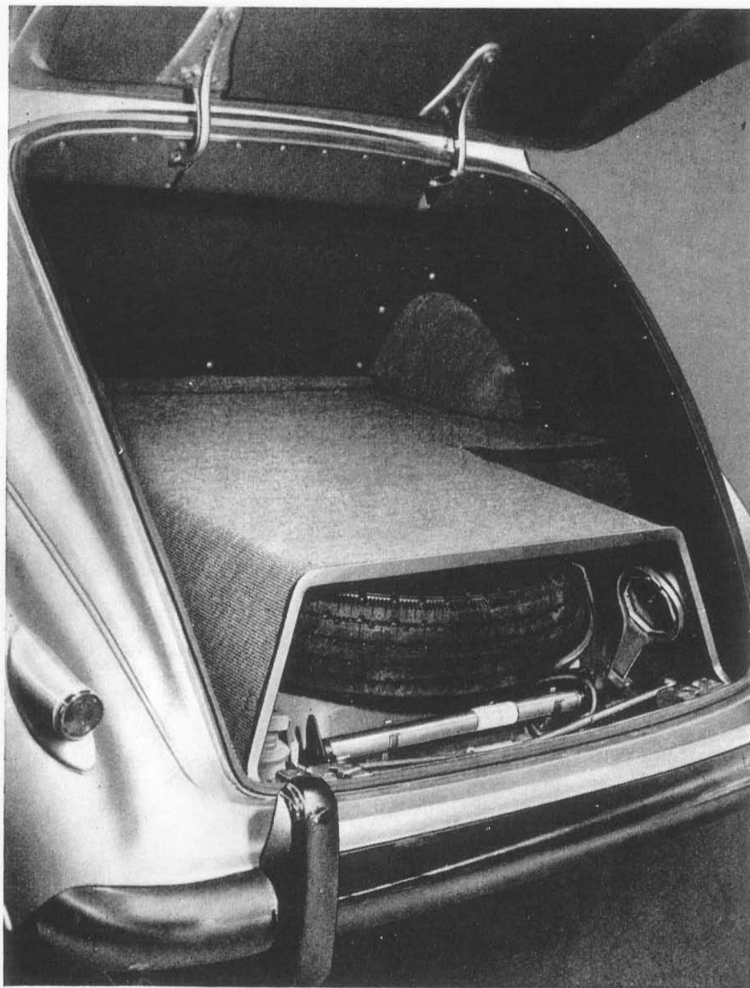
Fig. 56.—LUGGAGE BOOT, SPARE WHEEL AND TOOL COMPARTMENT.
