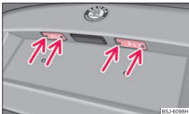
Fig. 174 Remove the licence plate light
