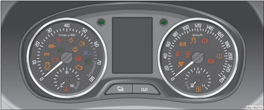
Fig. 22 Instrument cluster with warning lights
