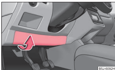
Fig. 161 Bottom side of the dash panel: Fuse cover
