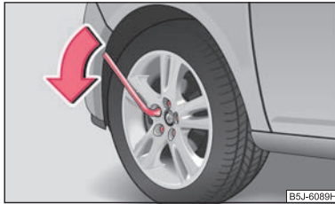
Fig. 154 Changing a wheel: Slackening wheel bolts
