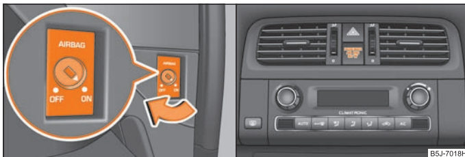
Fig. 121 Switch for the front passenger airbag / indicator light for a switched off front seat passenger airbag
