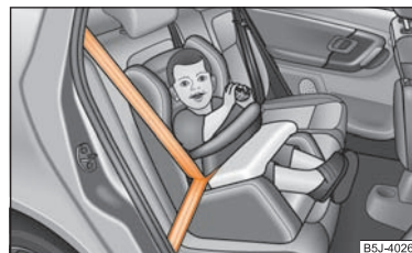
Fig. 125 Child seat with padded table in Group 1 installed on rear seat bench facing the direction of travel
