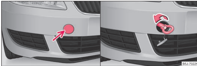
Fig. 159 Front bumper: Cover / installing the towing eye
