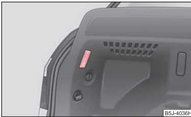
Fig. 177 Remove the luggage compartment light
