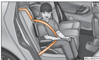
Fig. 126 Child seat in Group 2 installed on the rear seat facing the direction of travel
