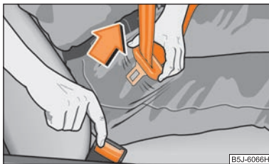
Fig. 113 Releasing lock tongue from belt lock
