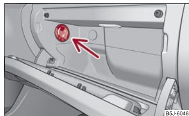
Fig. 80 Storage compartment: Using cooling system
