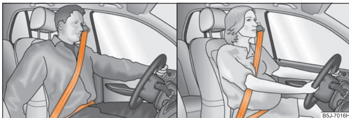
Fig. 111 Routing of belt webbing over the shoulders and the lap belt / Routing of belt webbing for an expectant mother
