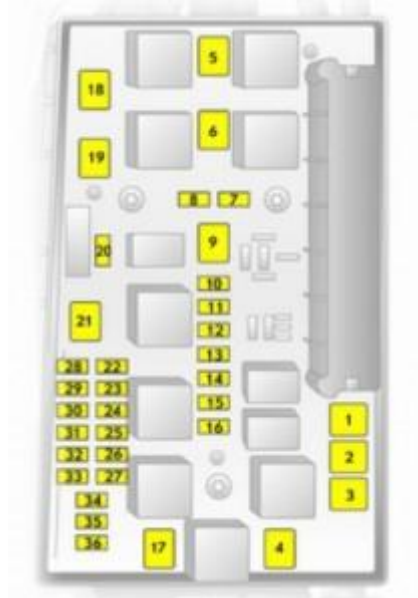
Vauxhall Zafira B – fuse box – engine compartment
