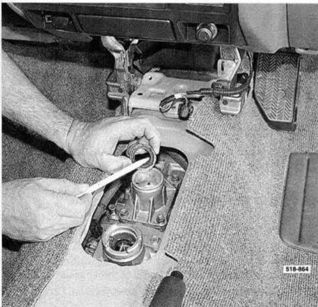
A cracked or deteriorated gear lever seat can cause a heavy and difficult gear change.
