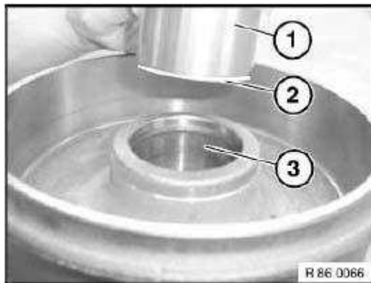
Fig. 103: Placing Wheel Bearing With Lathe-Turned End In Center Of Bore In Brake Drum Courtesy of BMW OF NORTH AMERICA, INC.
