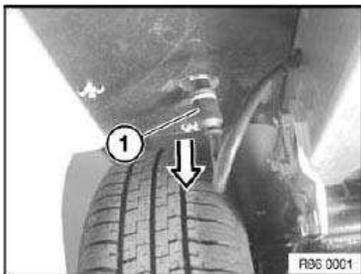
Fig. 106: Identifying Cable Tie
