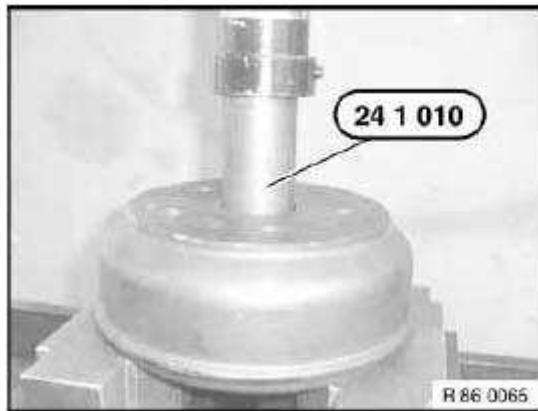
Fig. 102: Press Out Wheel Bearing With Special Tool 24 1 010 Courtesy of BMW OF NORTH AMERICA, INC.
