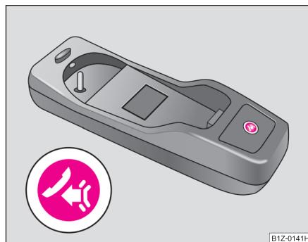
Fig. 100 Button for switching on the voice control
