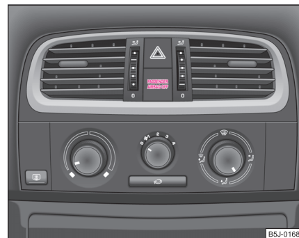
Fig. 122 Indicator light for a switched off front seat passenger airbag
