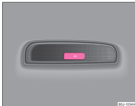
Fig. 42 Roof liner light at the rear
