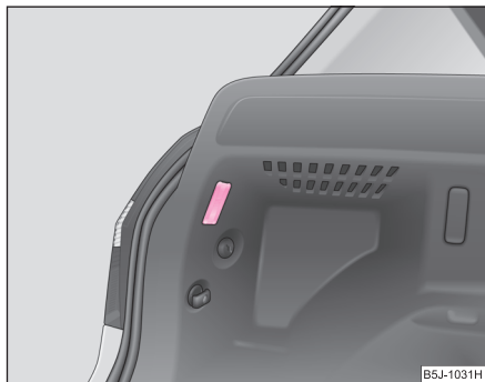
Fig. 181 Remove the luggage compartment light
