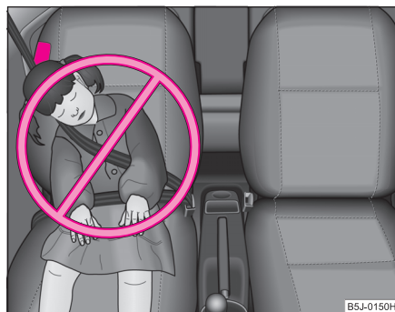
Fig. 124 Seated position of an unprotected child at risk from side airbag
