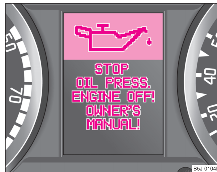
Fig. 13 Information display: Oil pressure is low
