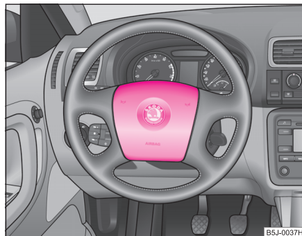
Fig. 113 Driver airbag in the steering wheel
