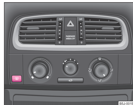
Fig. 43 Switch for rear window heater
