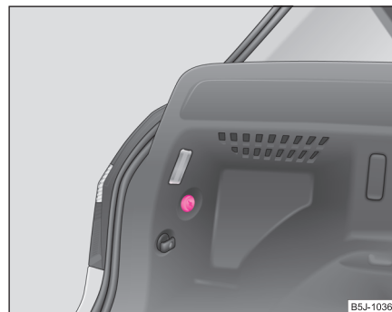
Fig. 178 Remove the rear light unit
