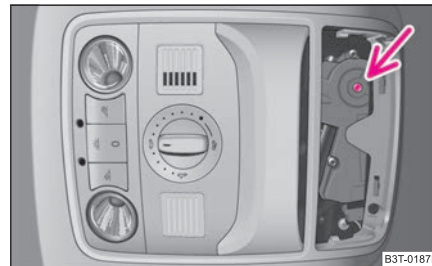
Fig. 40 Detail of the headliner: Emergency operation
