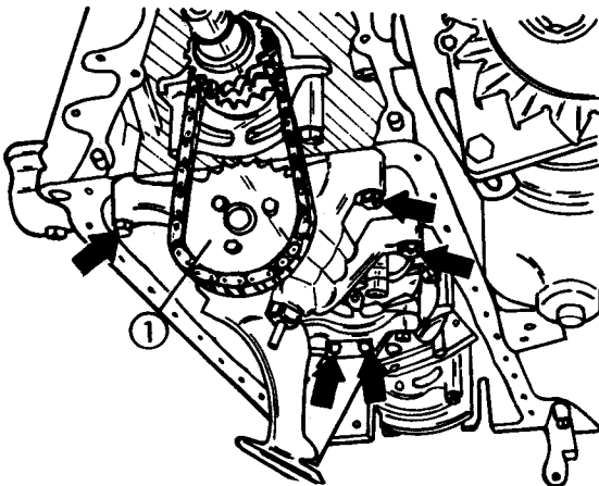
FIG 1:59 Oil pump and strainer removal
