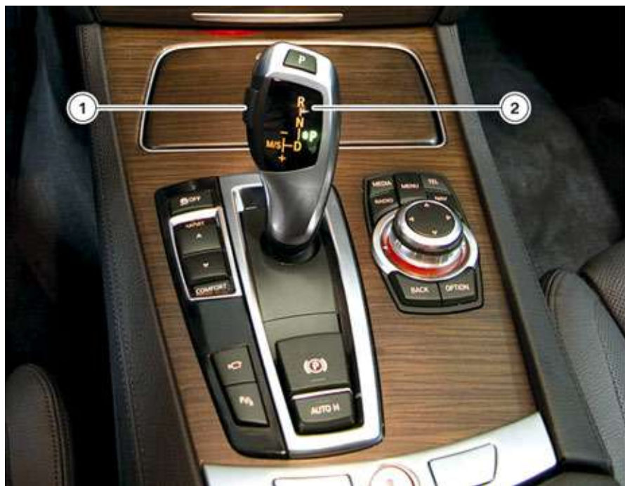
Electronic transmission emergency release GA8HP
