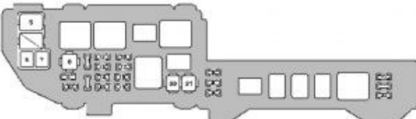
Lexus ES300 – fuse box – engine compartment
