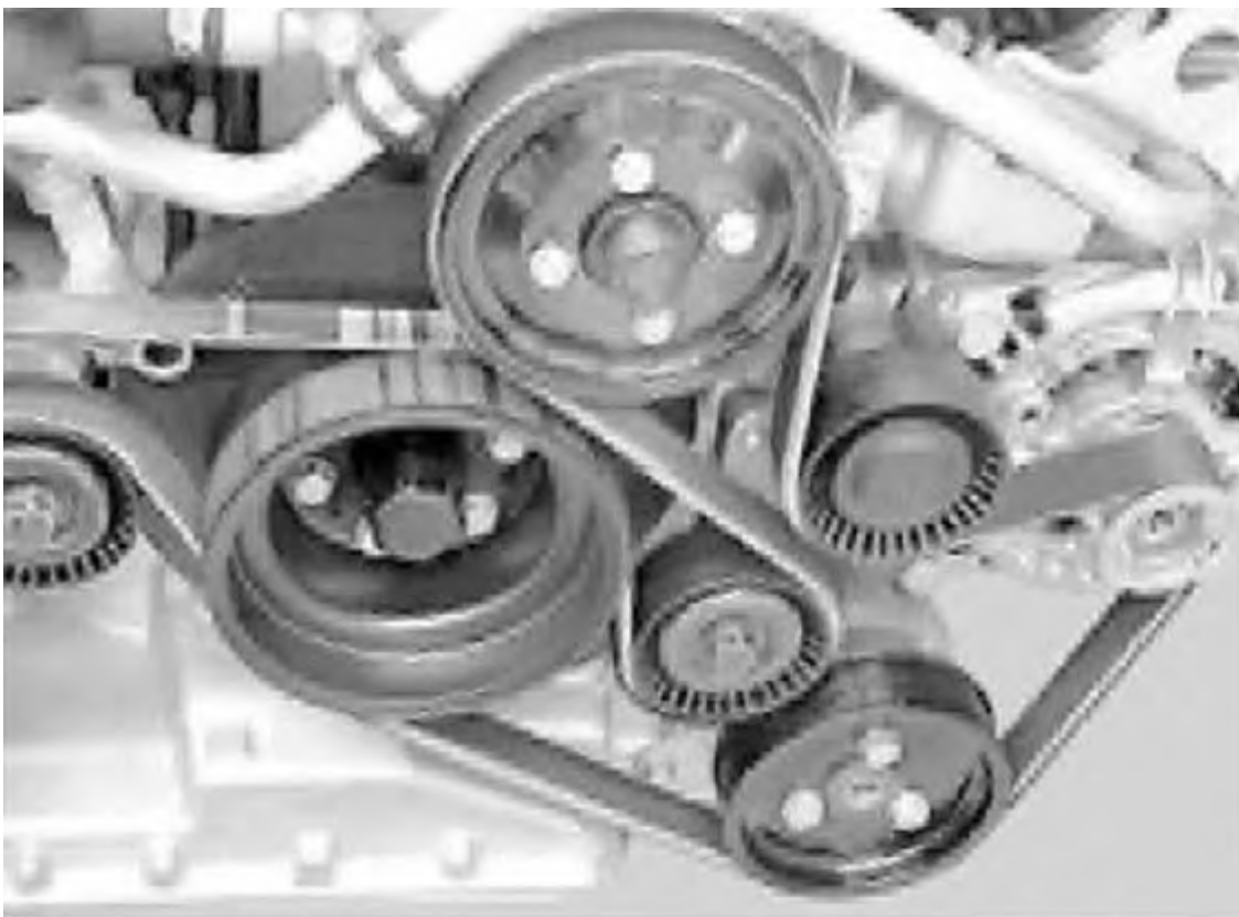
Fig. 45: Alternator Drive Belt Routing - 4.4L & 4.6L (M62) Courtesy of BMW OF NORTH AMERICA, INC.
