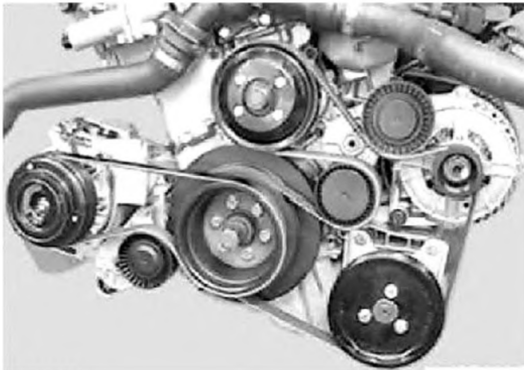
Fig. 42: Routing Alternator Drive Belt W/ Auxiliary Tension Roller - 3.0L (M54) Courtesy of BMW OF NORTH AMERICA, INC.
