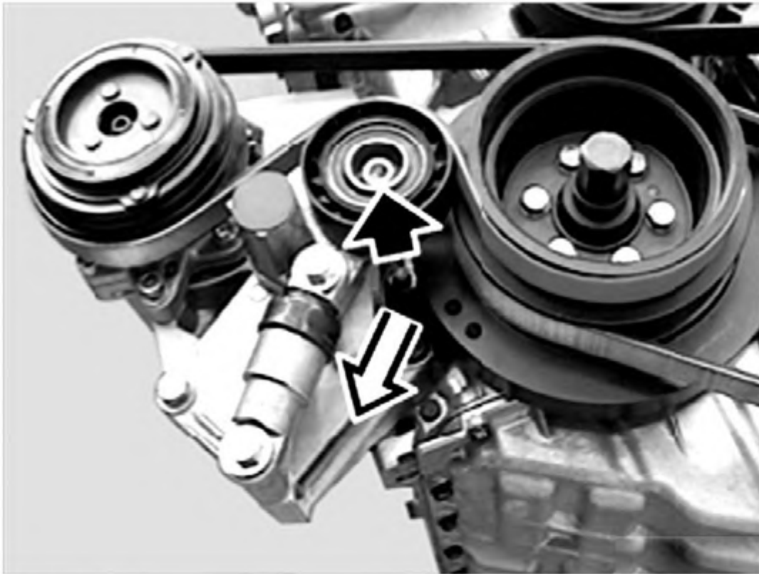
Fig. 8: Removing Hydraulic A/C Compressor Drive Belt - 3.0L (M54) Courtesy of BMW OF NORTH AMERICA, INC.
