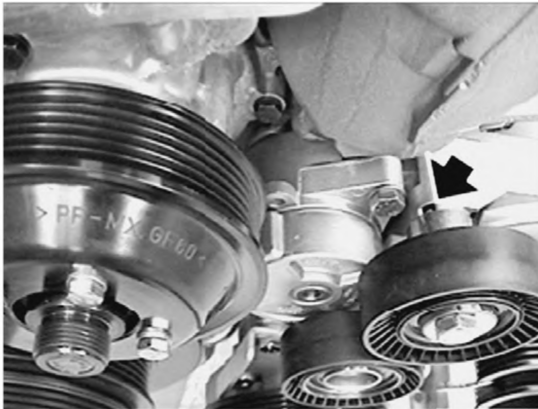
Fig. 43: Locating Locking Device Of Auxiliary Tensioning Roller - 3.0L (M54) Courtesy of BMW OF NORTH AMERICA, INC.
