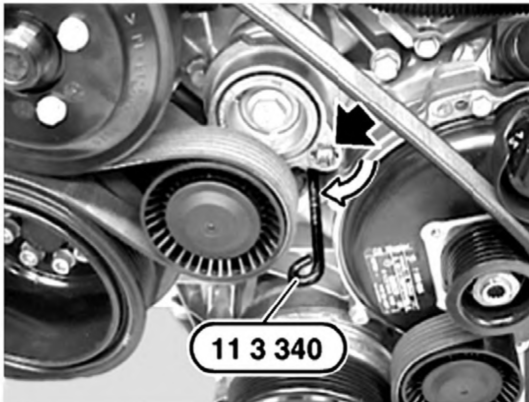
Fig. 47: Removing Generator Drive Belt - 4.4L (N62) Courtesy of BMW OF NORTH AMERICA, INC.
