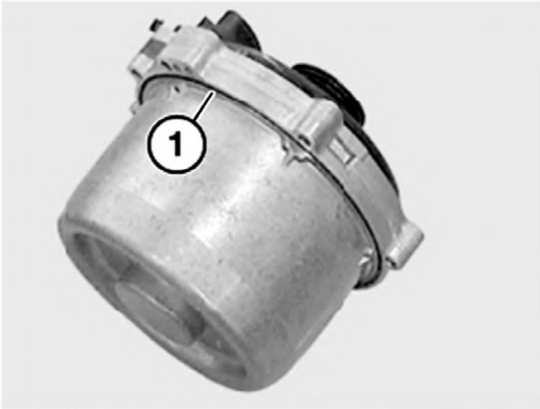
Fig. 32: Locating Sealing Ring - 4.4L & 4.6L (M62) Courtesy of BMW OF NORTH AMERICA, INC.
