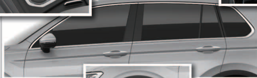
Door with exterior mirror mounted on shoulder line and side window
