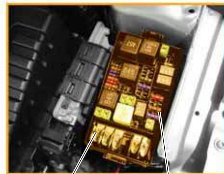
Multi-fuse pre-fuse holder SA on relay and fuse carrier SR1
