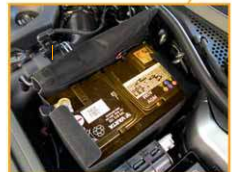
12-V battery in engine compartment There is no 12-V battery in the luggage compartment when the 12-V battery is fitted in the engine compartment.
