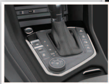
Operating unit for driving mode selection (4MOTION Active Control)
