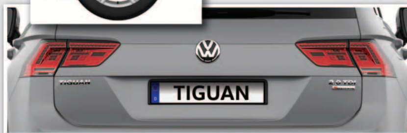
LED tail light cluster split into two sections with connecting character line
