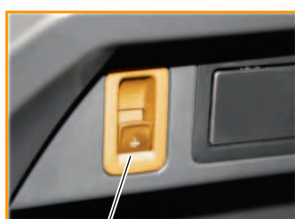
Electric hinged tow coupling attachment button E474
