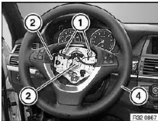
Fig. 62: Identifying Plug Connection, Steering Wheel And Screw Courtesy of BMW OF NORTH AMERICA, INC.
