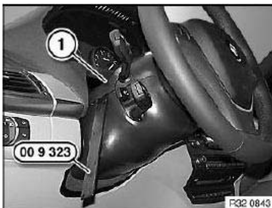
Fig. 51: Identifying Column Trim And Special Tool (00 9 323)
