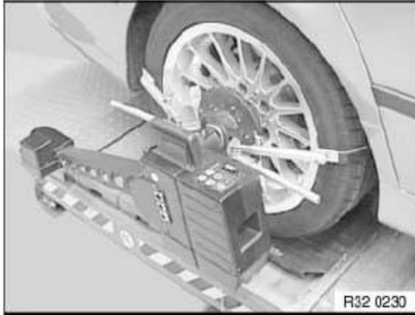
Fig. 17: Attaching Quick-Clamping Holder/Quick-Clamping Unit To Front Wheel Courtesy of BMW OF NORTH AMERICA, INC.
