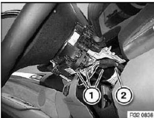
Fig. 54: Identifying Plug Connection And Wiring Harness Courtesy of BMW OF NORTH AMERICA, INC.
