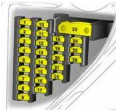
Vauxhall Signum – fuse box – passenger compartment
