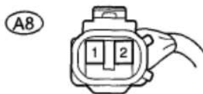
Fig. 38: Identifying Engine Hood Courtesy Switch Connector Terminals Courtesy of TOYOTA MOTOR SALES, U.S.A., INC.
