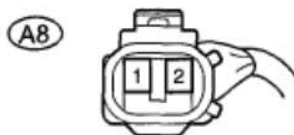
Fig. 12: Identifying Engine Hood Courtesy Switch Connector Terminals Courtesy of TOYOTA MOTOR SALES, U.S.A., INC.
