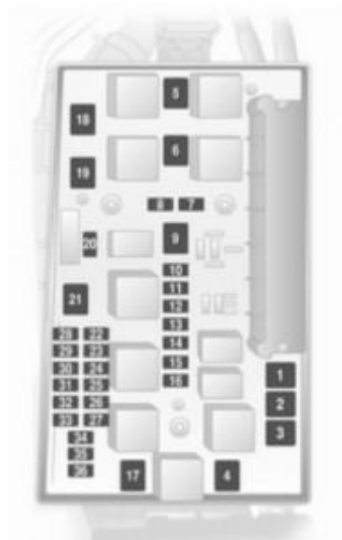
Vauxhall Astra (Astra J) – fuse box -engine compartment
