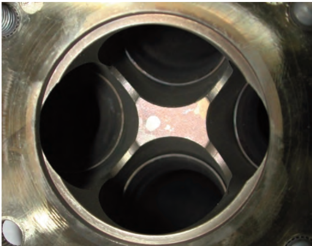
1 - Thin-wall tubular manifold with long single pipe routing for an optimum gas cycle.
