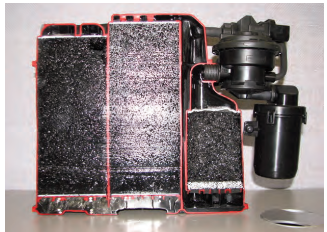
Inside view of Carbon Canister
