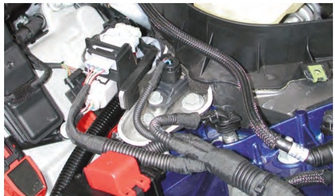
Body acceleration sensor on the left front.
