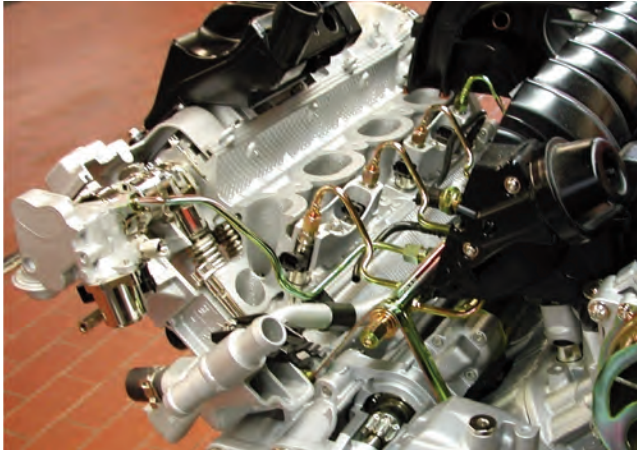
The picture shows the 3-piston high-pressure pump of the Panamera S
