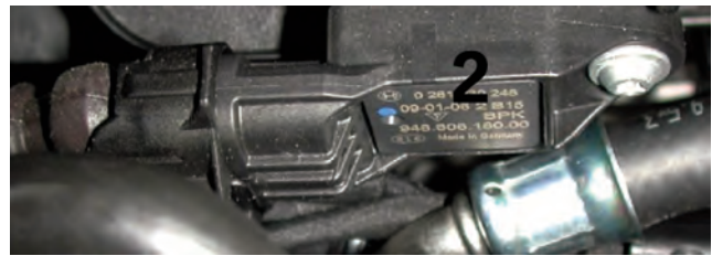
2 - Pressure sensor (at rear of intake manifold).
