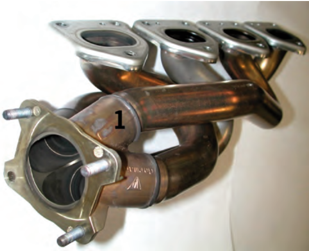
1 - Thin-wall tubular manifold with long single pipe routing for an optimum gas cycle.
