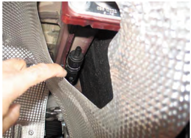
Air release damper left of the tank.
