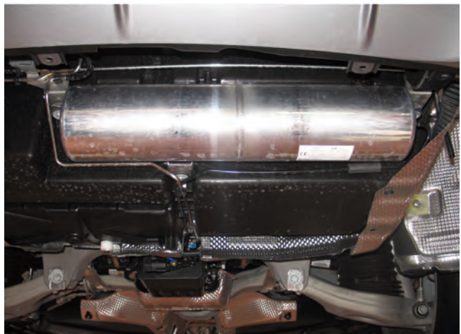
Pressure reservoir at the rear under the rear apron.
