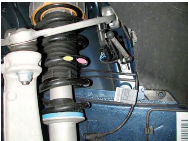
Color coding for suspension/chassis variant is shown in the above picture.
