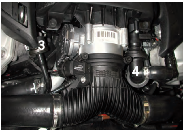
3 - Tank Vent Valve 4 - Positive Crankcase Ventilation
