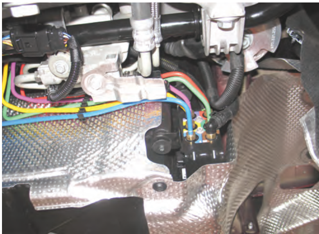
Valve unit - rear left, next to the compressor.
