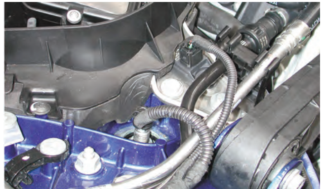
Body acceleration sensor on the right front.
