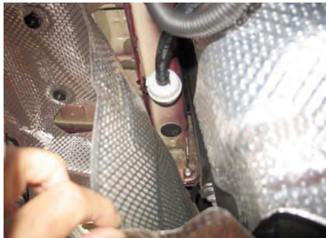
Installation position of intake air filter - right of the tank.
