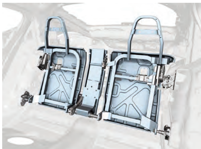
Lightweight backrest structure in aluminum.
