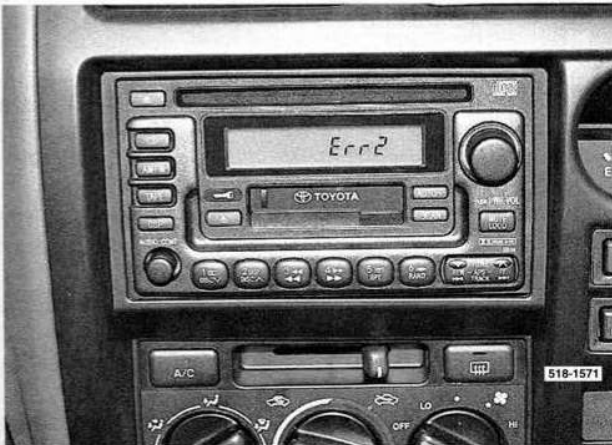
The display panel shows the number of errors made entering the security code.
