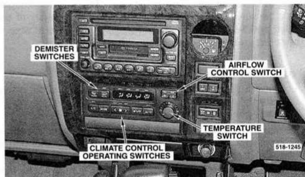
Climate control panel switches installed.
