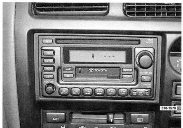
When these symbols on the display panel appear, the sound system security code can be entered.
