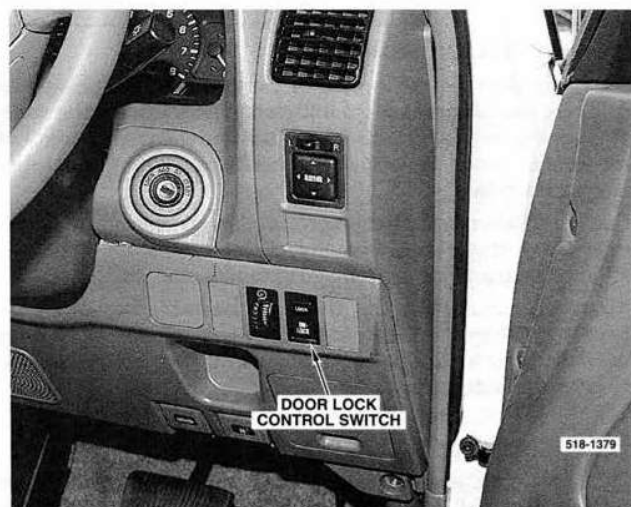
On model without power windows the door lock switch is located on the lower dash panel.
