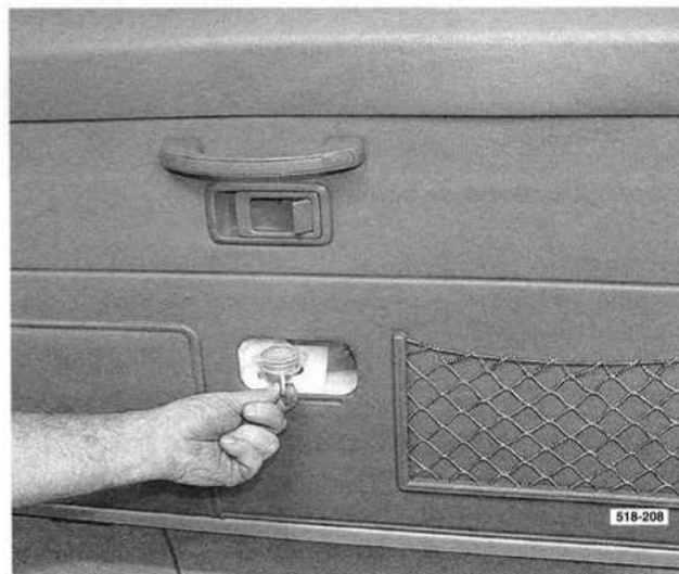
Preparing to fill the tailgate washer bottle.
