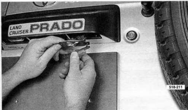
Removing the number plate lamp assembly.
