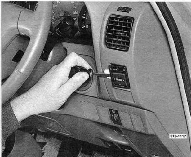
Removing the power mirror switch from the instrument panel.
