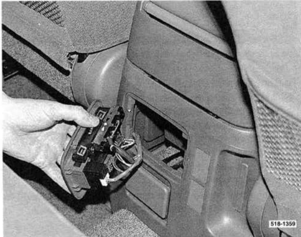
Removing the climate control panel from the rear of the centre console.
