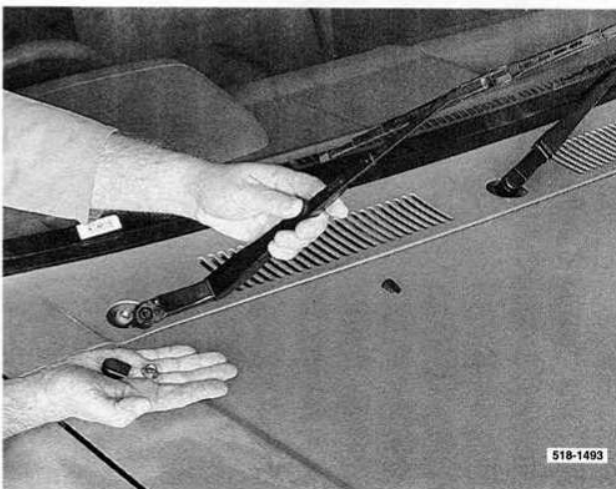
Removing the windscreen wiper arm.
