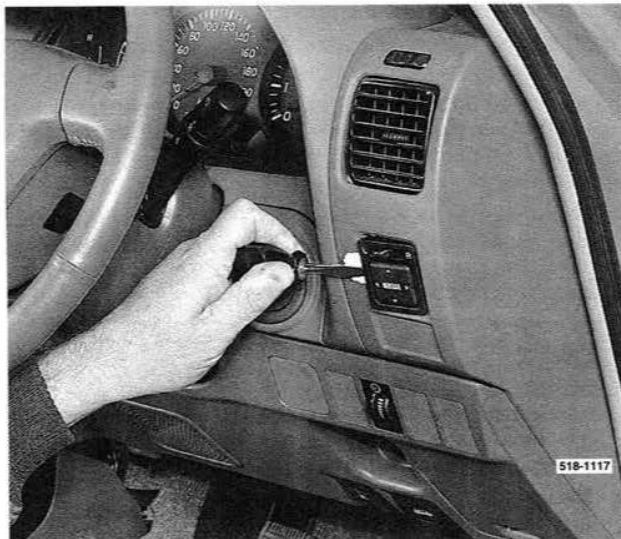
Removing the power mirror switch from the instrument panel.
