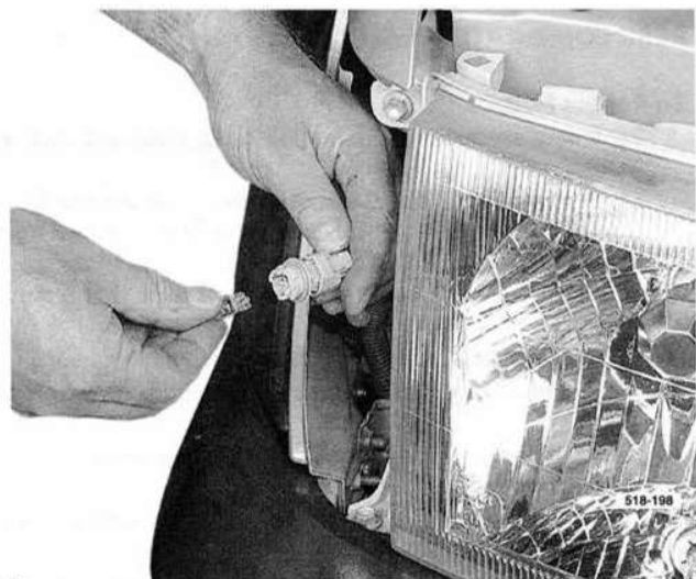
Removing the park lamp bulb.
