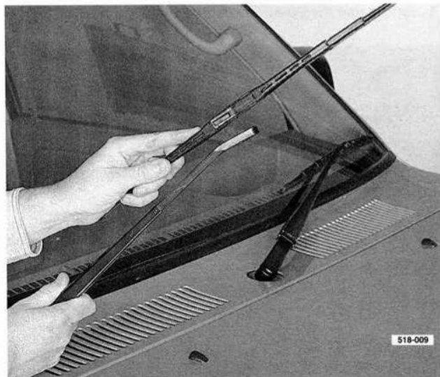
Removing the wiper blade from the wiper arm.
