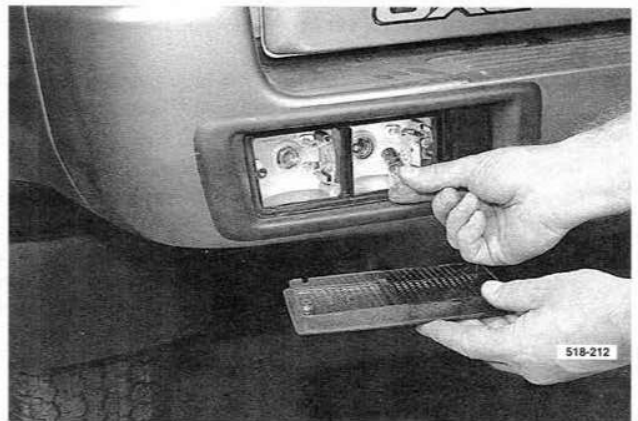
Removing the lower combination lamp bulb.
