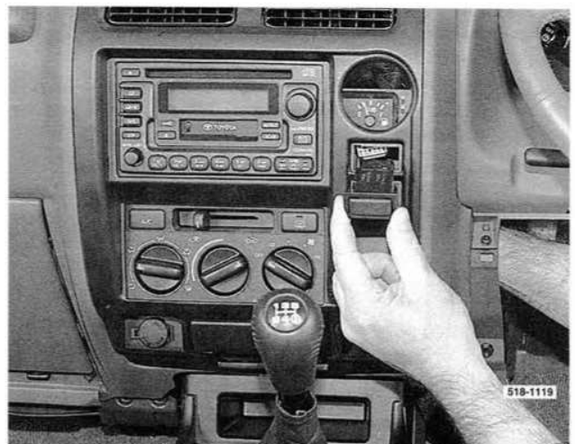
Removing the switches from the radio surround panel.
