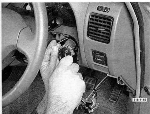
Removing the lock cylinder from the lock housing.
