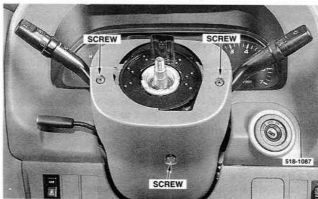
Location of the steering column cover retaining screws.
