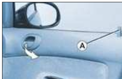
Opening the doors from inside
