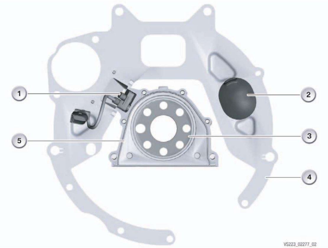
Fig. 4: Position of crankshaft sensor
