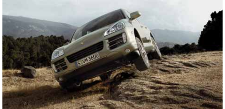
PDCC in on-road mode: reduced wheel articulation
