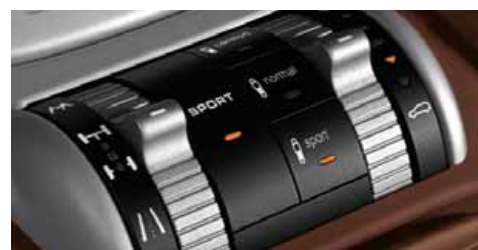
PASM control with 'Comfort', 'Normal' and 'Sport' options
