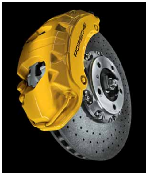
Porsche Ceramic Composite Brake (PCCB), front disc diameter: 410 mm
