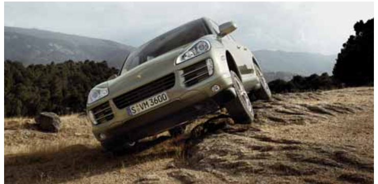
PDCC in off-road mode: increased wheel articulation
