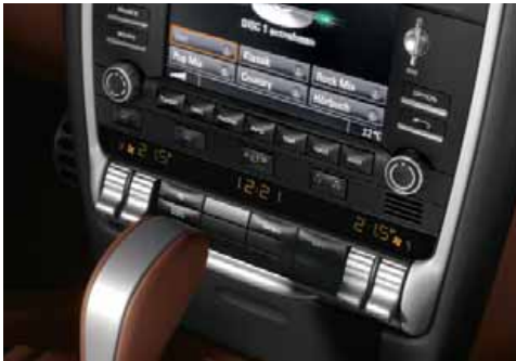
Air-conditioning controls (cover open)
