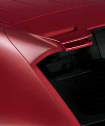
Extended roof spoiler with fixed bi-plane wing elements
