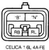
Fig. 11: Park/Neutral Switch Terminal ID (1.6L 4A-FE) Courtesy of Toyota Motor Sales, U.S.A., Inc.
