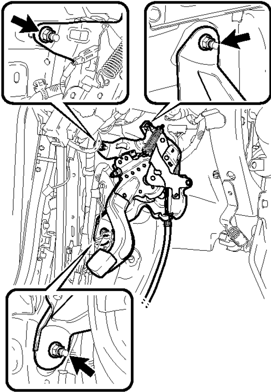
Fig. 73: Identifying Parking Brake Control Pedal Assembly & Fasteners Courtesy of TOYOTA MOTOR SALES, U.S.A., INC.
