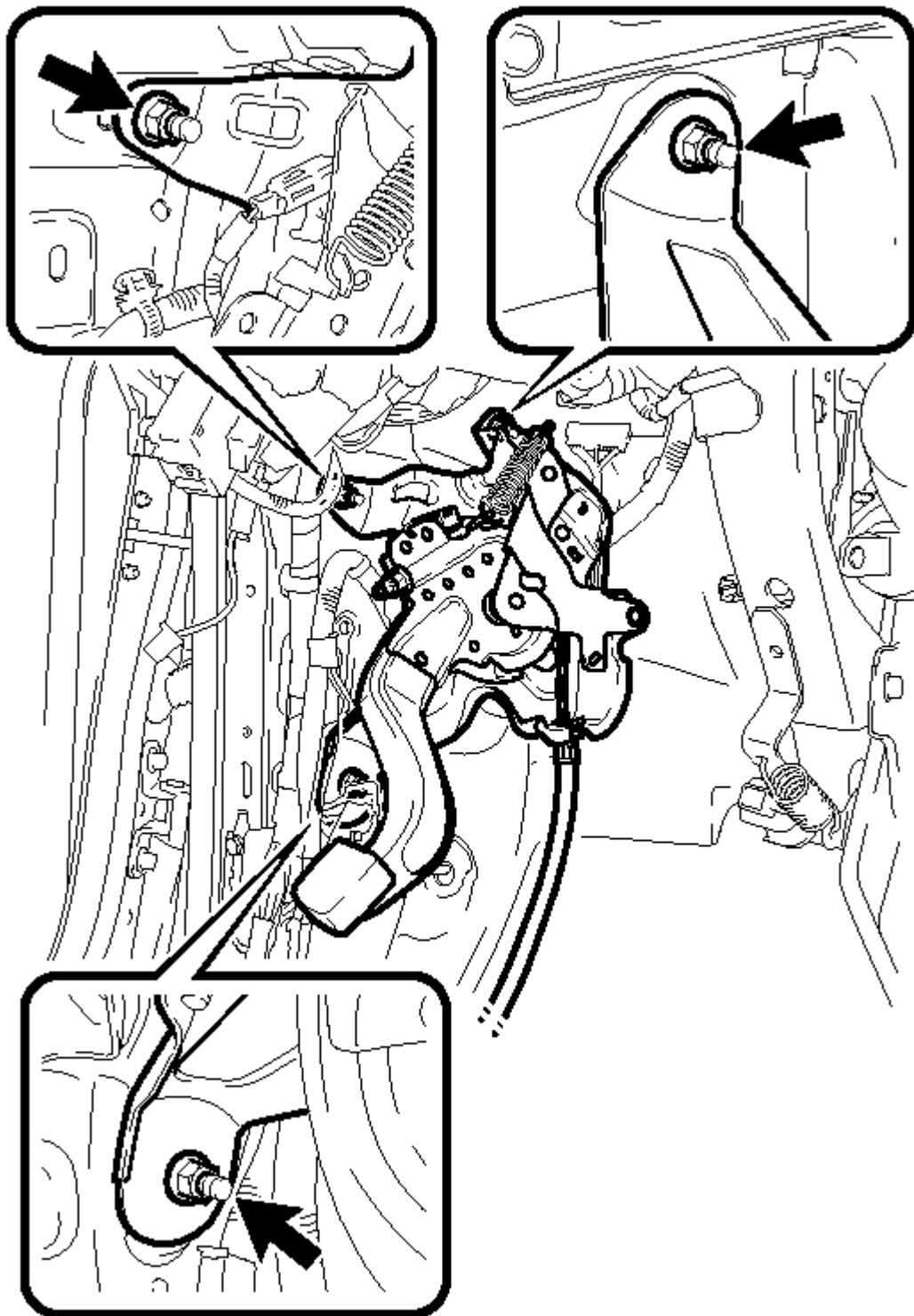
Fig. 16: Identifying Parking Brake Control Pedal Assembly & Fasteners Courtesy of TOYOTA MOTOR SALES, U.S.A., INC.
